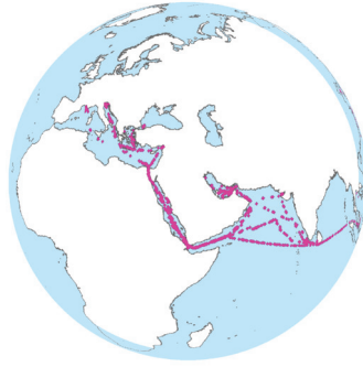
Figure 3: Track of a vessel reconstructed from both terrestrial and satellite AIS data over the course of the year 2012. Data: LuxSpace Sarl. (satellite) and JAKOTA Cruise Systems (terrestrial).
